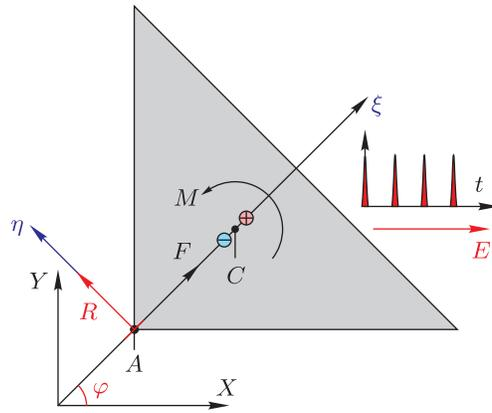
**Fig. 1.** Chaplygin sleigh under the action of force  $F$  and torque  $M$ . The knife edge attached at point  $A$  is oriented as shown by the red segment. The center of mass  $C$  is located at distance  $a$  from the knife edge on the axis  $\xi$ . The laboratory reference frame  $(X, Y)$  and the frame fixed relatively to the sleigh  $(\xi, \eta)$  are used.
