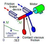
Fig. 1. A system of two Froude pendulums: the motion of one and the other pendulum is decelerated alternately by attaching a brake shoe providing suppression of the selfoscillations
