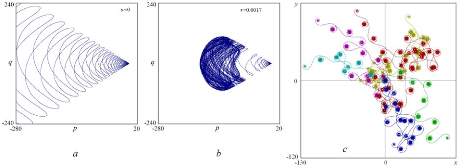
Fig.1. Unbounded acceleration of the sleigh (a) and bounded acceleration where the trajectory approaches a chaotic attractor (b) accompanied by random-like walk in the laboratory frame (c). Parameters are  $a=0$ ,  $I_0 = 0.15$ ,  $\mu = 0.85$ ,  $\nu_1 = 0.35$ ,  $\nu_3 = 0.1$ ,  $\varepsilon = 1$
